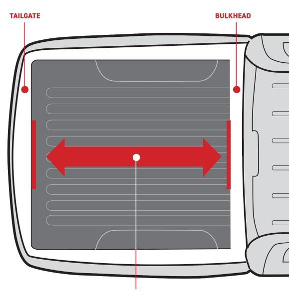
Measure from inside of tailgate to inside of bulkhead.
